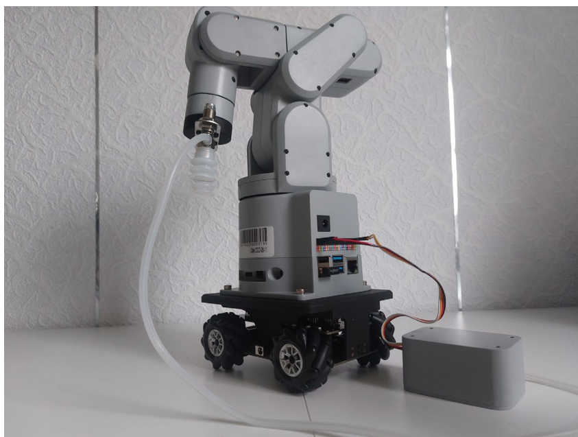
Fig.1 Brațul robotic Mecharm Pi
